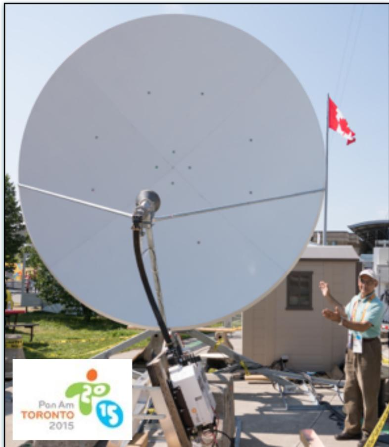
**Antenna features linear or circular C-band feed horns and redundant SSPB transmitters**
